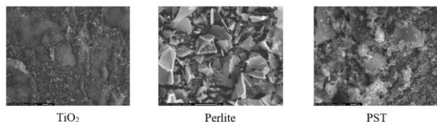
Figure 4. SEM images of TiO 2 (5000X), perlite (1000X), and PST (5000X) samples [11].
