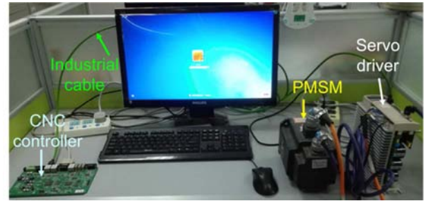
Figure 3. Experimental apparatus for repetitive position control of PMSM.
